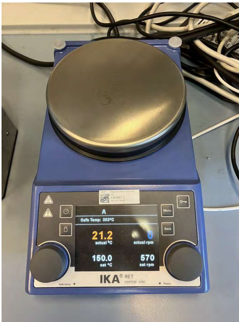
Figure 10. Hot plate for annealing.
