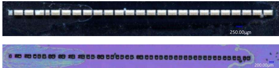
Figure 10 Fused-silica compound refractive lens
