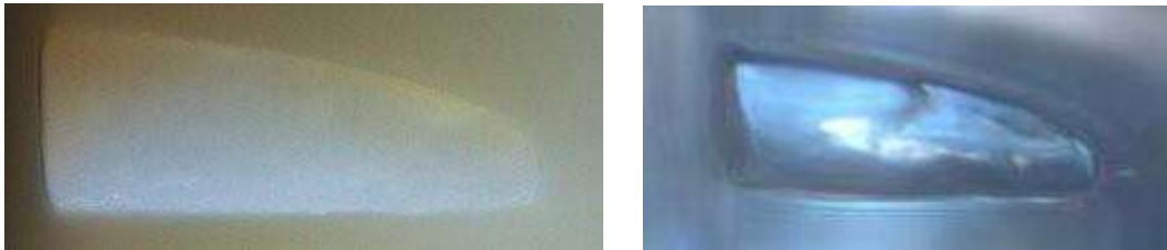
Figure 8 Structural change from green part to final structure after sintering process
